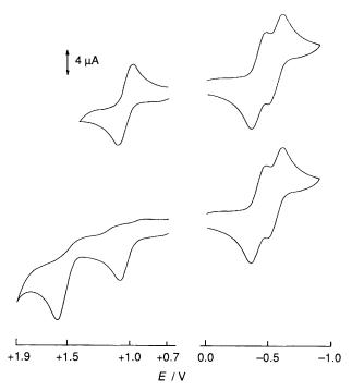
Figure 1. Cyclic voltammograms of (1), 0.1 mM in PhCN-0.1 M  $Bu_4NCIO_4$  at room temperature (scan rate: 50 mV s<sup>-1</sup>; reference electrode: SCE). A: Swept at the potential range from -1.0 to +1.4 V; B: from -1.0 to +2.0 V.
